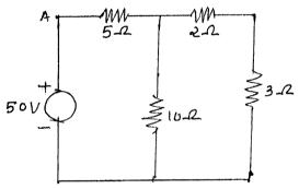
(B) Write the statements of Tellegen's and Millman's theorems. Verify the reciprocity theorem for the following circuit:
